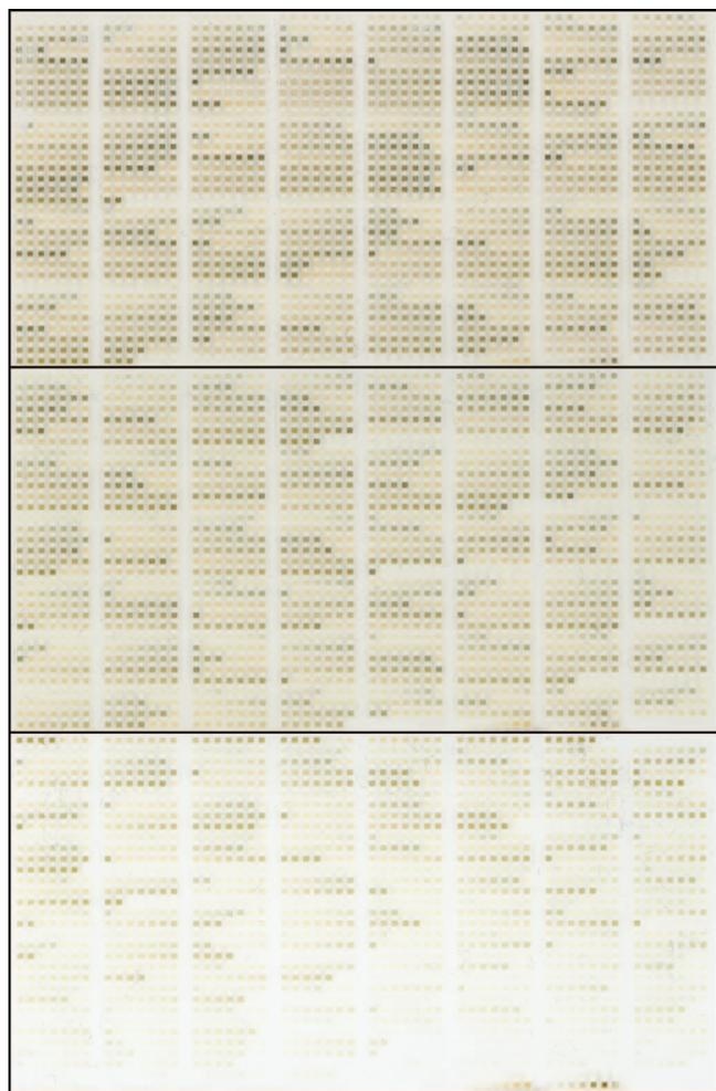
**Figure 1.** Images of the 3 plates containing the 5456 samples in the (Fe-Co-Ni-Ti) $O_x$  library. The thin film samples are each 1 mm square and are arranged on a regular grid on the FTO coated glass plates.
