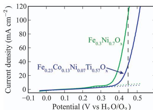
**Figure 2.** Results from the electrochemical scanning voltage measurement are shown for two samples, each from a composition region of high OER catalytic activity. For each anodic voltage sweep, a linear residual current (dotted line) is automatically identified, from which the OER catalytic current is measured. The catalytic current at 450 mV overpotential (dashed line) is used to compare activity across the composition library.
