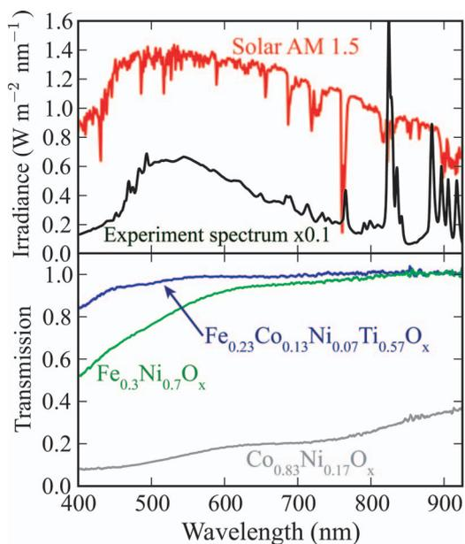
**Figure 3.** (top) The AM1.5 solar irradiance and the optical experiment irradiance are shown over the wavelength range used for characterization of catalyst transparency. (bottom) Transmission spectra for the catalysts of Fig. 2 are shown along with the spectrum for the least transparent catalyst.
