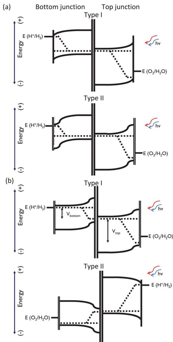
**Fig. 1** Schematic energy band diagrams of an integrated photoelectrochemical (PEC) system under 1 Sun illumination for (a) the photocathode + photoanode PEC system, denoted as Configuration A, and (b) the tandem light absorber + electrocatalyst PEC system, denoted as Configuration B. Types I and II illustrate the semiconductor–liquid junctions and buried junctions, respectively, as described in the text.
