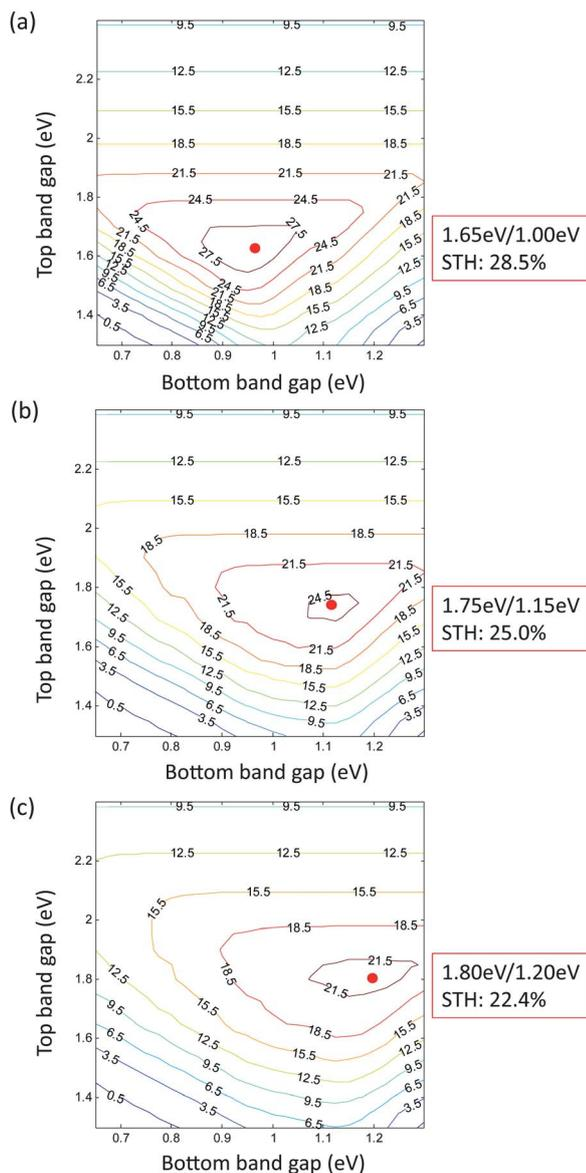
**Fig. 6** Iso-efficiency plots of the STH efficiency limits for a series of light absorber fill-factors (FFs), (a) FF = 0.85, (b) FF = 0.75, and (c) FF = 0.68. State-of-the-art earth-abundant catalysts, such as NiMo and NiFeO<sub>x</sub>, were chosen as the HER and OER catalysts, respectively, and the solution resistance was 5 ohm cm<sup>-2</sup>.
