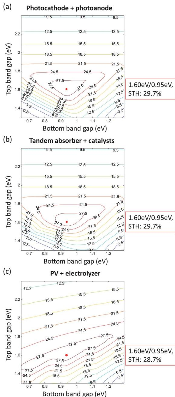
**Fig. 3** Iso-efficiency plots showing the STH efficiency limits for (a) a photocathode + photoanode PEC, (b) a tandem absorber + electrocatalyst PEC, and (c) a two-junction PV + electrolyzer. In (a) and (b), Pt and RuO<sub>2</sub> were chosen as the HER and OER catalysts, the light absorber had FF = 0.85, and the solution resistance was 5 ohm cm<sup>-2</sup>. In (c), the electrolyzer efficiency was taken to be 73%.
