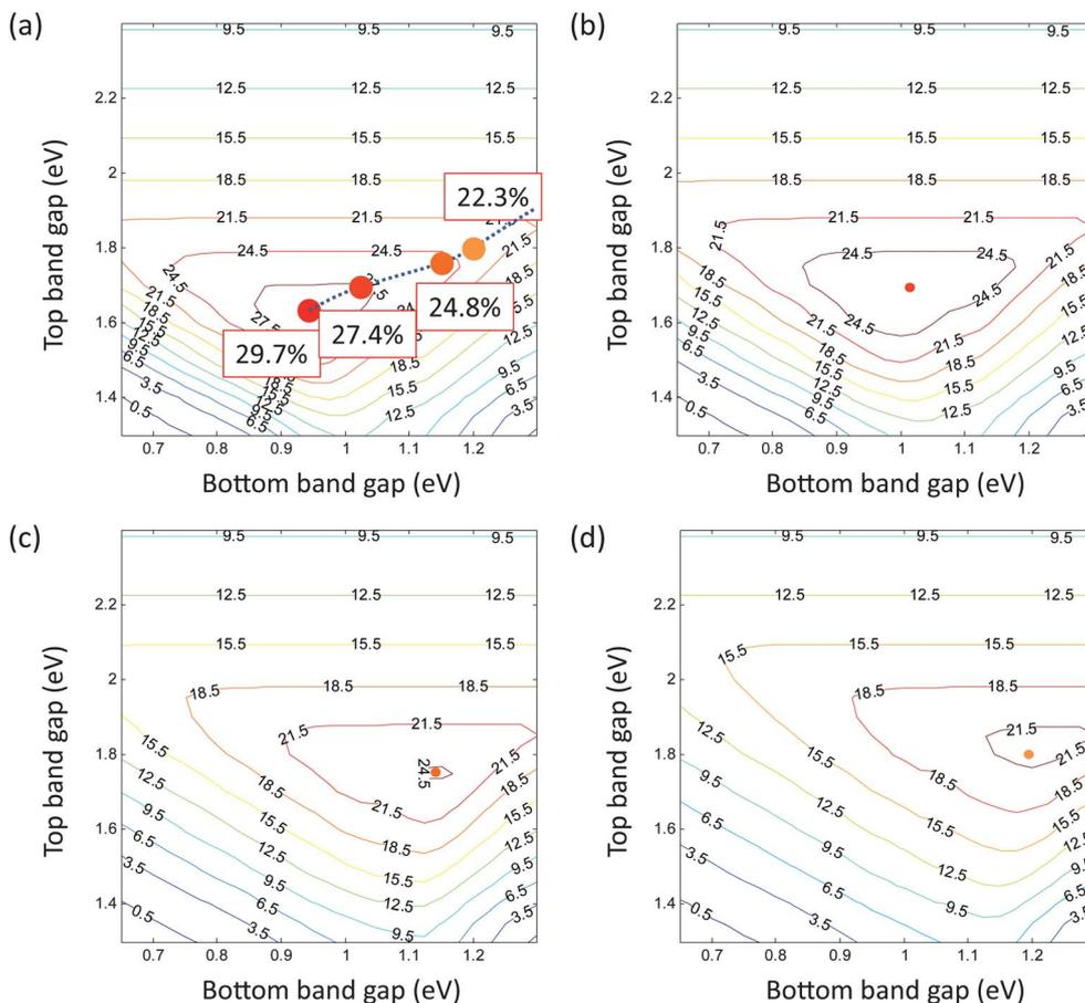
**Fig. 5** Iso-efficiency plots of STH efficiency limits for a series of solution resistance values of: (a) 5, (b) 10, (c) 20, and (d) 30  $\text{ohm cm}^{-2}$ . The dots in (a) represent the maximum STH efficiencies for  $R = 5, 10, 20,$  and  $30 \text{ ohm cm}^{-2}$ , with the traces varying as a function of the solution resistance value labeled as the dashed line. Pt and  $\text{RuO}_2$  were chosen as HER and OER catalysts, respectively, and the light absorber had a  $\text{FF} = 0.85$ .
